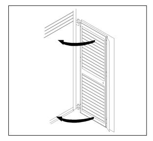
• Close the external securing flap so that it clamps onto the roller shutter curtain.
