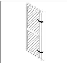
• Pull the door and frame back away from the roller shutter so that it is completely clear of the curtain, and locate it back to the wall with either the locating pin or hook and eye.
