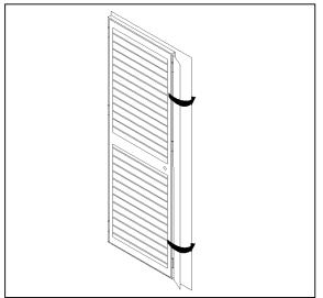
• Turn the top and bottom internal levers to lock the external securing flap.
