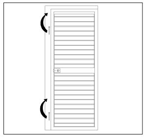
• Swing out the external securing flap to release the door from the roller shutter curtain.
